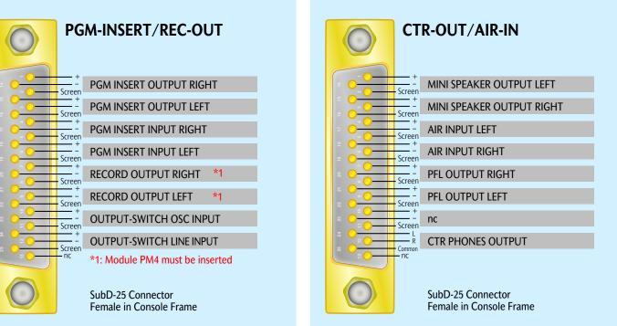
switch input. When using the internal oscillator, a cable from the oscialltor output jack has to be installed.
