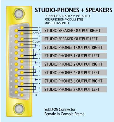
dio speakers outputs of the playback module BC-STU4b. While the studio speakers outputs are standard, electronically balanced, line level outputs, the headphone outputs are unbalanced to drive headphones directly. Each output can drive approx. 3
