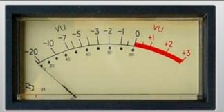
and default to and adjustment to 0 dB VU @ 0 dBV (+ 4 dBV with 4 dB lead) equivalent to  $\sim$  + 2 dBu. The adjustment range covers all commonly used settings. The VU meters are available in panels with 2 or 4 meters. Two meters are 80 mm / 2 module compartments wide.
